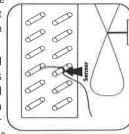
between an entrance point and outgoing point of the refrigerant tubing. In case of any doubt, measure the condensing temperature and select the point which is closest to the saturation point.
